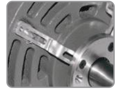
AEGIS® EP2400 Conductive Epoxy installation
