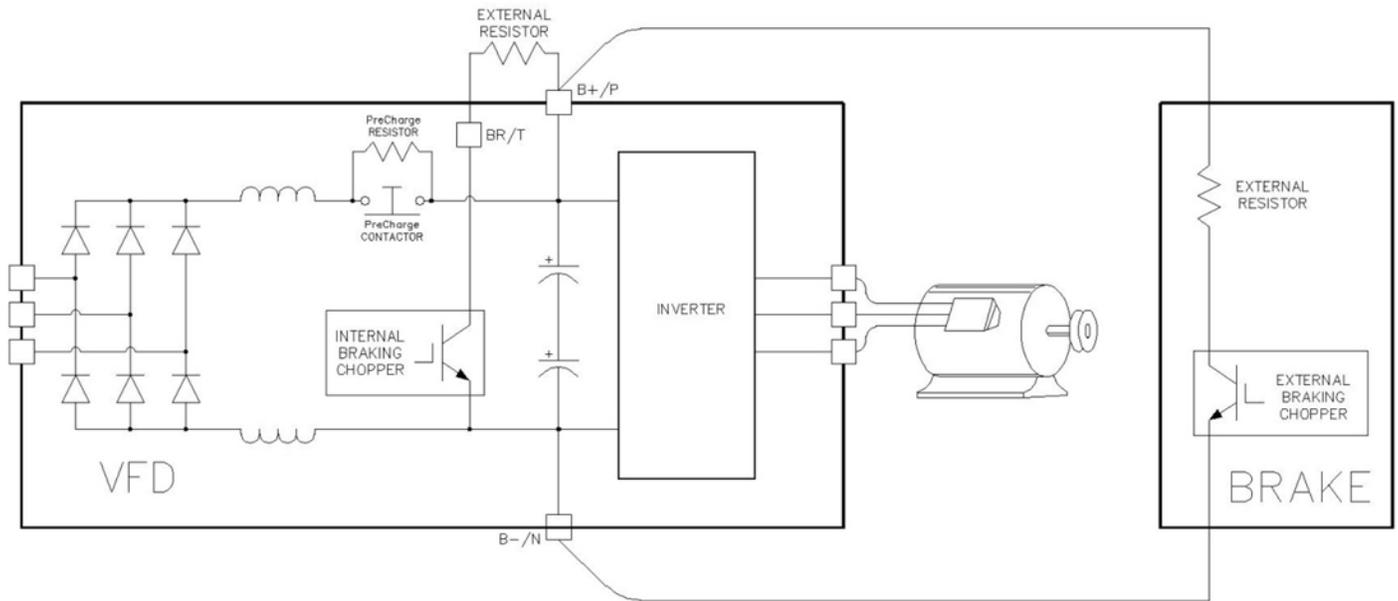
**Internal/External Chopper:** In the example above, the internal and external chopper connections are shown. Both should never be used at the same time. An external chopper is needed when a drives internal chopper cannot support the desired duty cycle, or when the drive has no internal chopper transistor.
