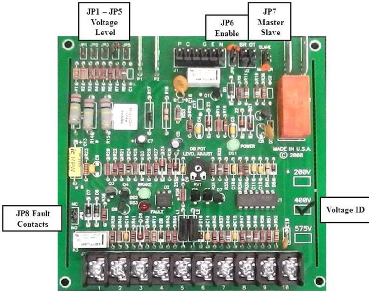
**FIGURE 4b: Control Board Jumper Positions**
