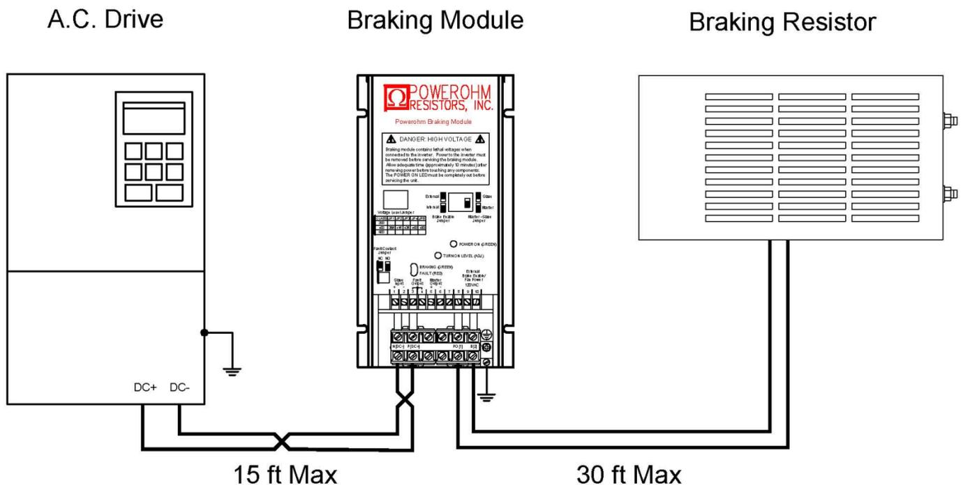
**WARNING: Never install a braking resistor directly across the DC bus of the drive. Drive damage or failure may occur upon applied power or, the resistor will dissipate power continuously and be subject to overheating and failure.**
