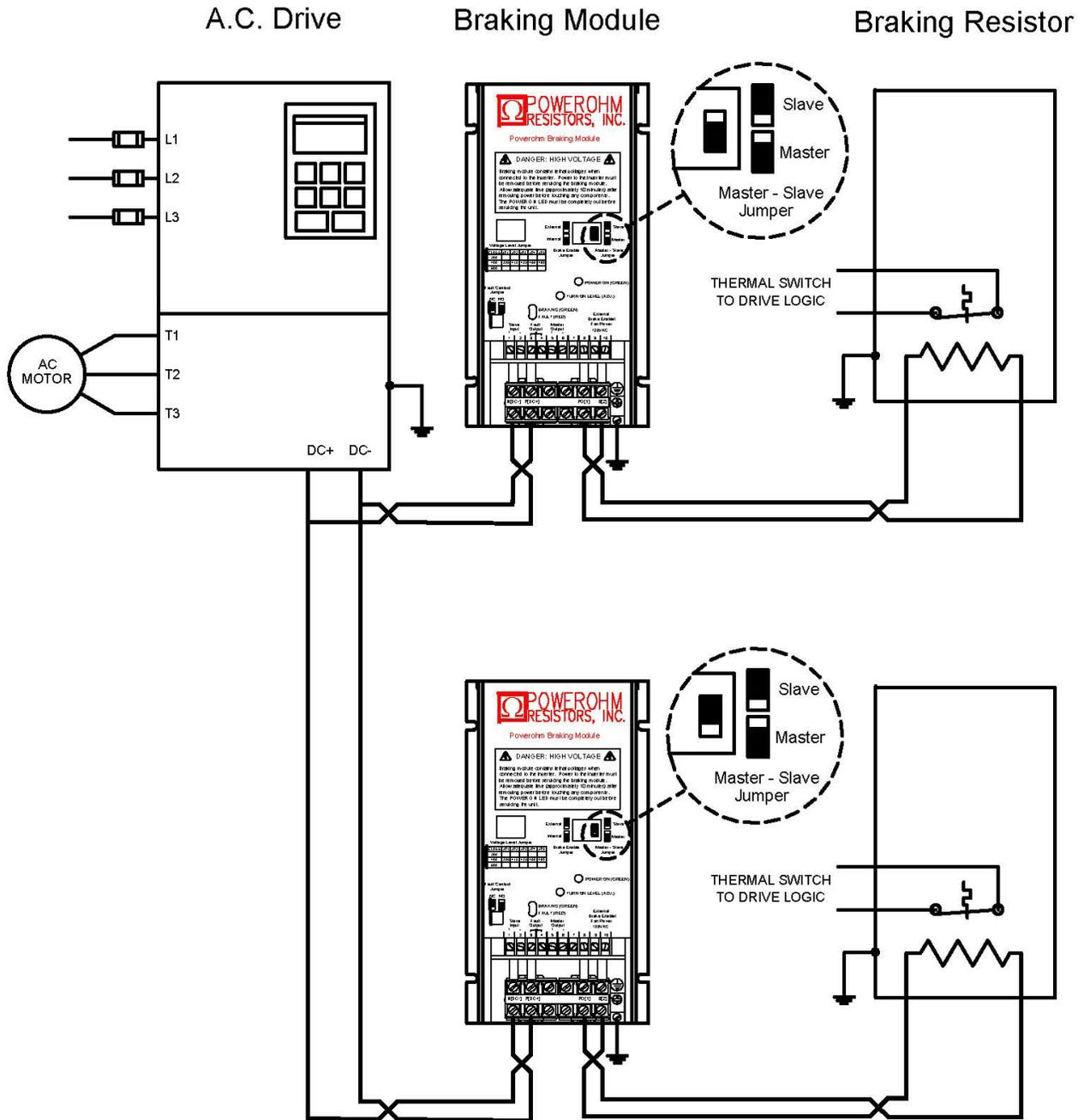
**Master - Slave Jumper Settings:** In the example above, the top braking module is set as the Master (JP7 is the downward position) and the lower module is in Slave Mode (JP7 is in the upward position).
