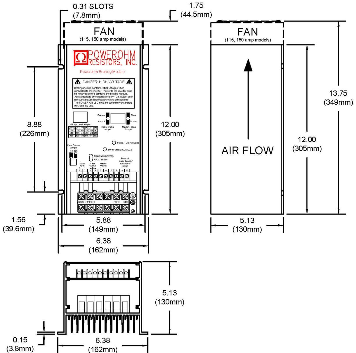
**Weight:** For 50amp the weight is approximately 9 lbs; For 115 & 150 amp the weight (with fan) is approximately 11 lbs.
