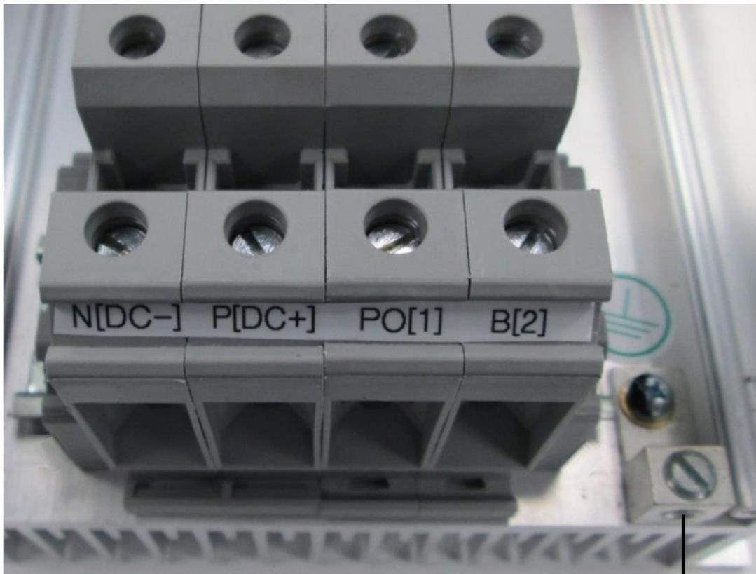
The PowerOhm Series UBU Braking Module features a 10-position terminal block for all signal and control wiring. All terminations on the block can accept bare wire or fork lugs for a #6 screw. Reference Table 4 for a description of each terminal.
