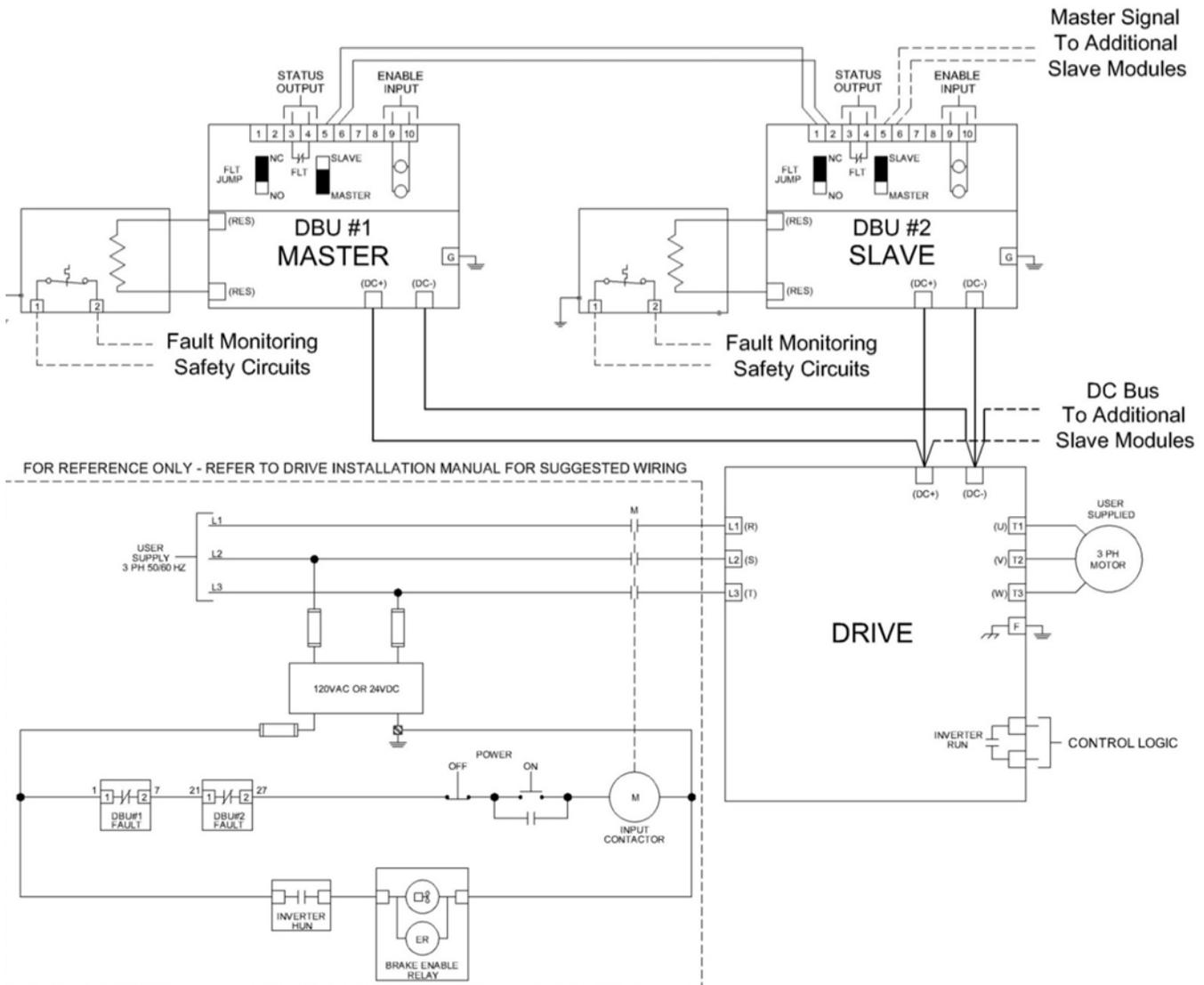
**Master - Slave Jumper Settings:** In the example above, the top braking module is set as the Master (JP7 is the downward position) and the lower module is in Slave Mode (JP7 is in the upward position).
