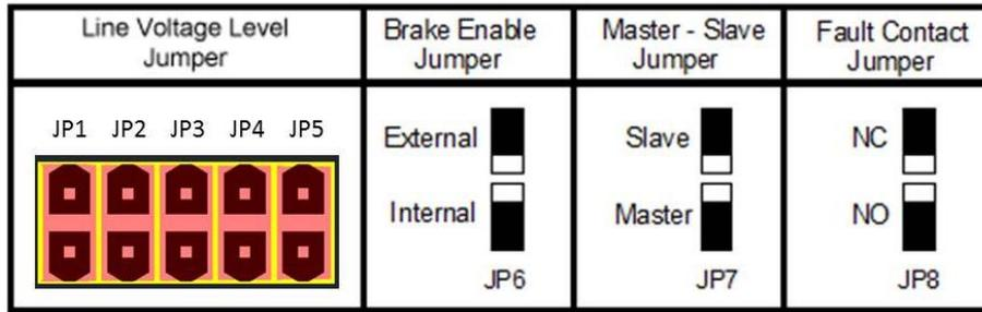
**Brake Enable Jumper:** JP6 selects between internal enable or external enable modes
