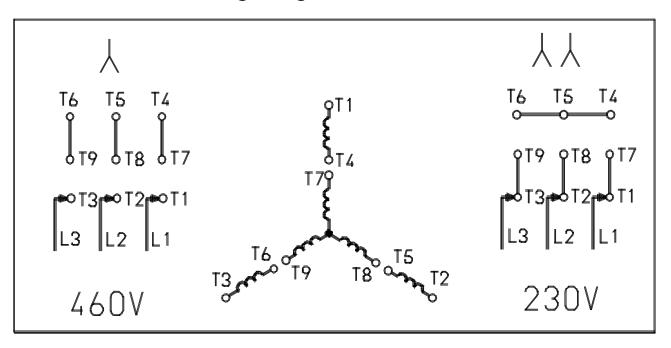
To reverse direction of rotation interchange connections L1 and L2.
