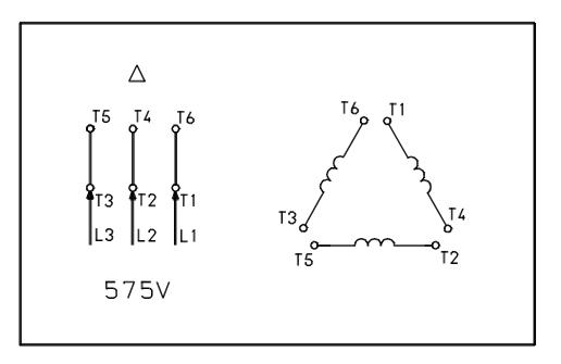
To reverse direction of rotation interchange connections L1 and L2.
